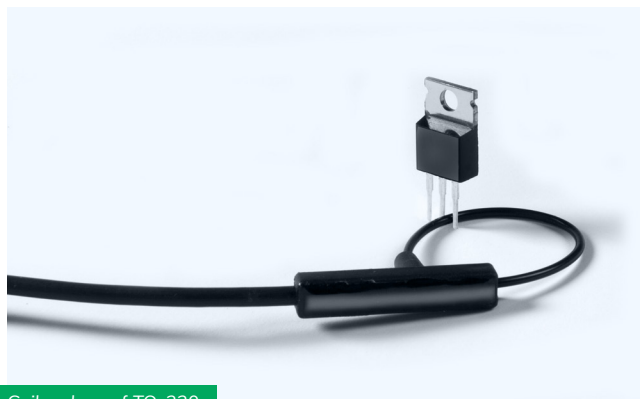
Coil on legs of TO-220
