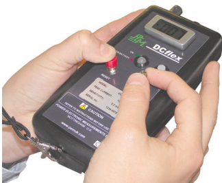
Press the reset button. Null the offset trimmer to zero
