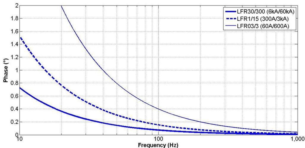
Figure 3. LFR Phase response 10Hz to 1kHz bandwidth
