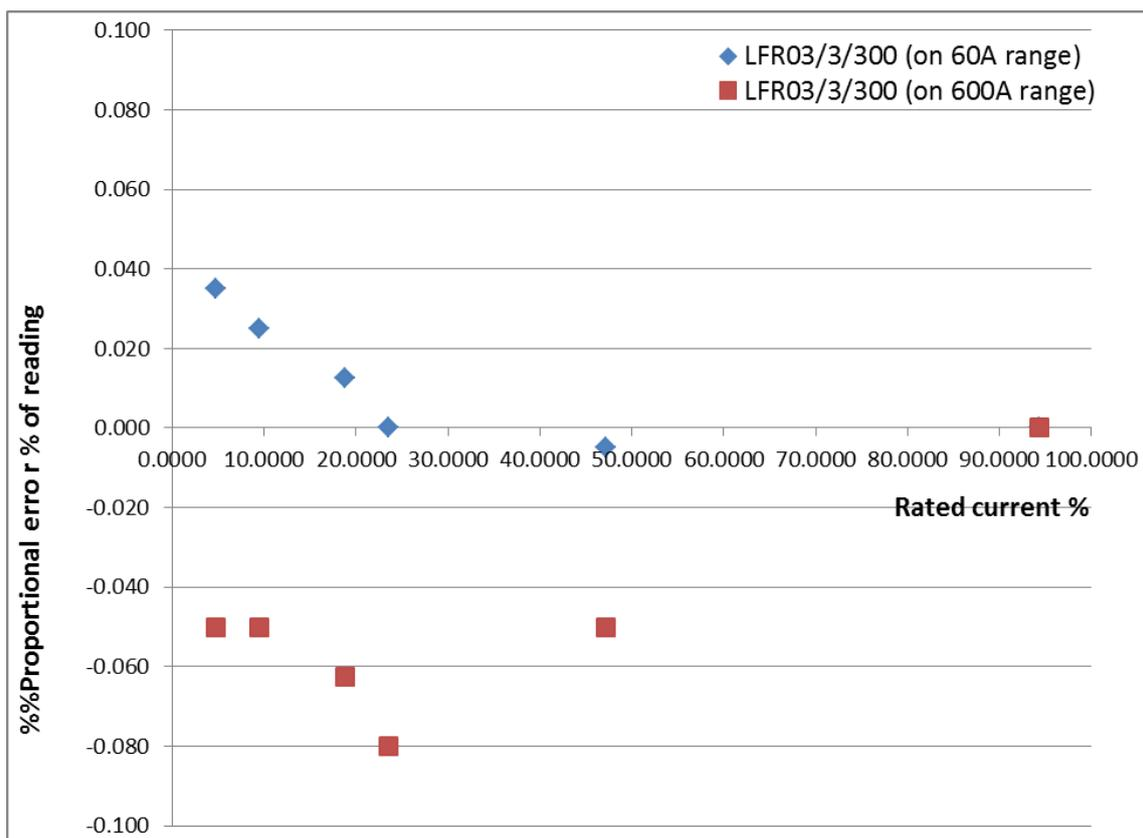
**Figure 6. Linearity of the LFR03/3 with 300mm coil**
