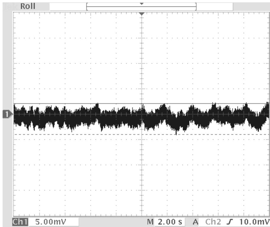
**Figure 7. Noise on 10mV/A (600A peak range) LFR03/3**
