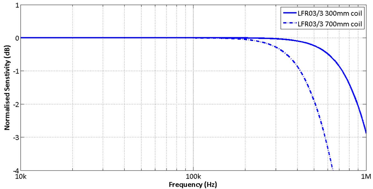
Figure 4. A comparison of the amplitude response > 10kHz of LFR 03/3 with a 300mm coil and a 700mm coil.
